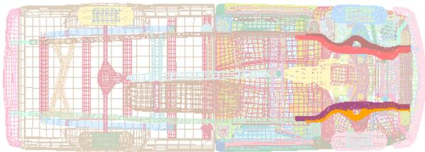
Figure 3: Bottom view of the finite element model of a pick-up truck. The four longitudinal chassis beams shown in the right of the figure need to be partitioned into regions with similar bending behavior in a series of crash simulations.
