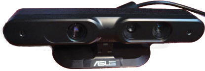
Figure 4: The user controls position and orientation of the virtual object by moving one hand in front of a depth camera.
